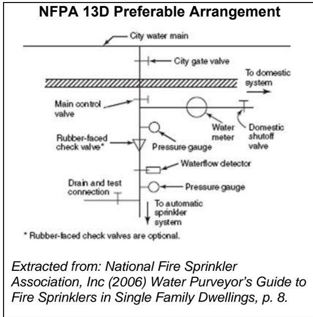
System configuration options provided in NFPA Standard 13D allow sprinkler system flow to be either metered or not metered. For example, this diagram shows Standard 13D's Preferable Arrangement for a sprinkler system with regard to the water meter, while 13D also shows two other "Acceptable Arrangements" in which the sprinkler flow is metered (National Fire Sprinkler Association, Inc 2006).
